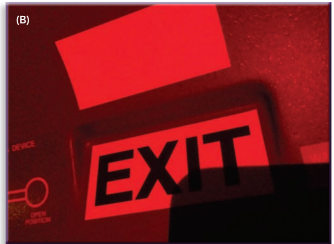
FIGURE 2 Example of complete “disappearance” of red letter print on a white background under dimmed red light conditions. The two photographs show the same section of the medical (passenger) compartment of our Airbus H-135 HAA helicopter. (A) Taken in daylight. (B) Taken in darkness, illuminated by a commercial head lamp (Black Diamond®) in red light mode.
