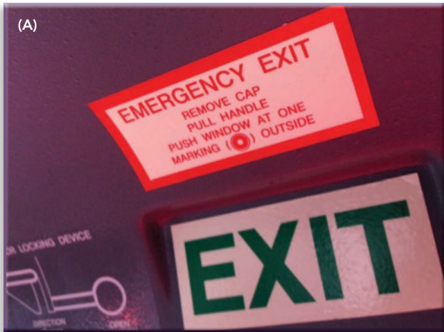
FIGURE 2 Example of complete “disappearance” of red letter print on a white background under dimmed red light conditions. The two photographs show the same section of the medical (passenger) compartment of our Airbus H-135 HAA helicopter. (A) Taken in daylight. (B) Taken in darkness, illuminated by a commercial head lamp (Black Diamond®) in red light mode.
