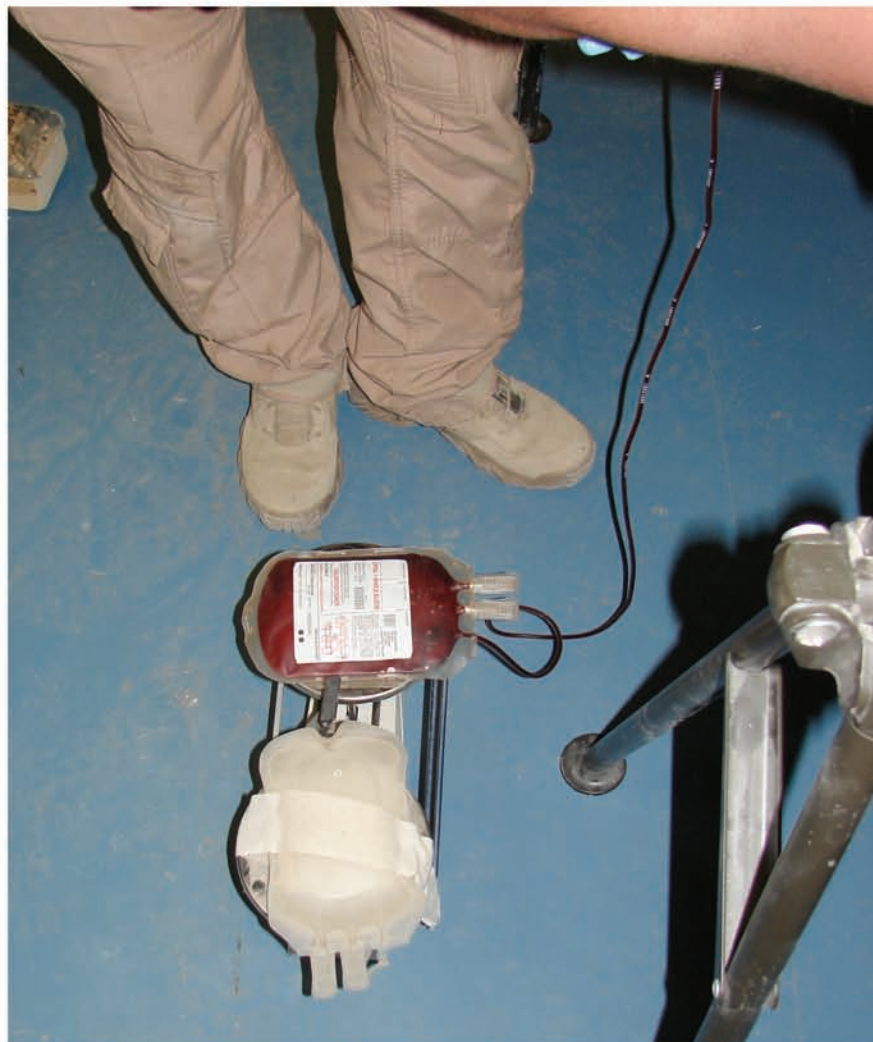
Blood Trip Scale Made from a Balance Beam Scale with Improvised Counterweight (Photo courtesy LTC Shawn C. Nessen, MD)
