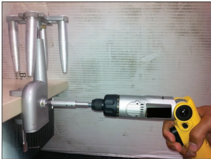
Hand Cranked Centrifuge Connected to Cordless Drill Using Locally Manufactured Adapter
