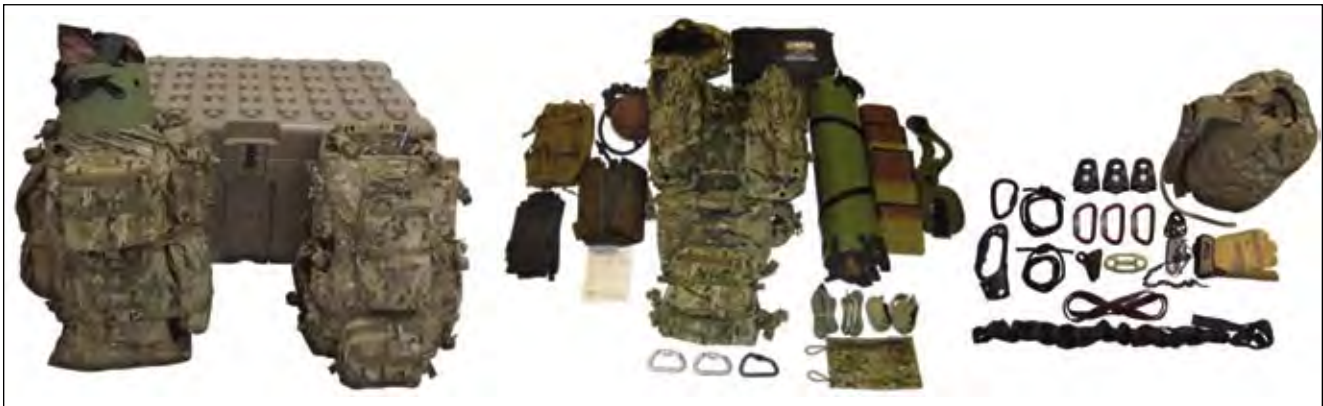
Modules E-1 and E-2 provide all necessary equipment for horizontal and vertical patient rigging and lifts along with harnesses and tools for personnel fall protection/prevention.
