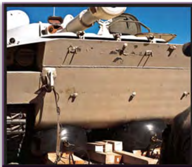
During field testing, the E3 module was used to conduct a point lift of a M109 Paladin (27.5 tons!).
