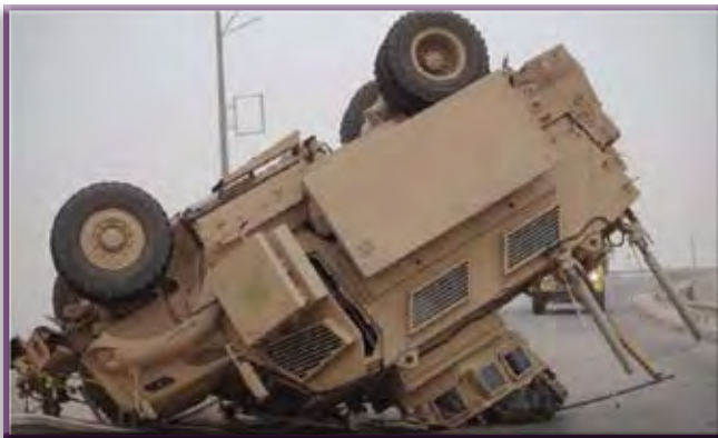
Rollover incidents create multiple rescue obstacles to include, casualty access, extrication, and fire suppression.
