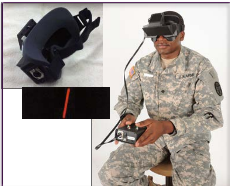
Figure 2 An example of a simple field test for vestibular function developed recently by Dr. Andrew Clarke and colleagues of the Charité Medical School of Berlin and being evaluated by the authors of this report. This is a portable, automated version of the subjective visual vertical test, which detects unilateral otolith dysfunction (unilateral deficit can cause inability to orient a line vertically).
