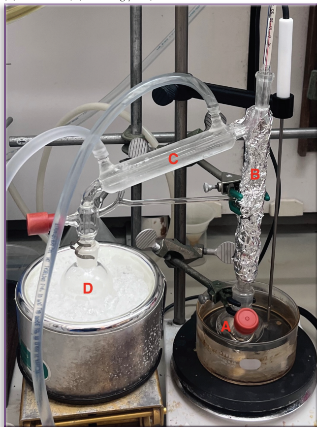
FIGURE 1 Image of equipment for the acid-catalyzed dehydration of ethanol to form diethyl ether and the fractional distillation of the diethyl ether. (A) 50mL flask in which sulfuric acid was added to a solution of ethanol. (B) distilling column, containing a thermometer. (C) condenser. (D) receiving flask, in an ice bath.
