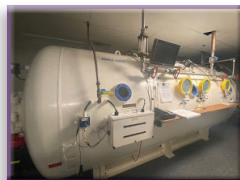
FIGURE 4 Dual-lock/multi-place recompression chamber at the National Oceanic Atmospheric Administration (NOAA) in Seattle, WA.
