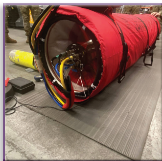
FIGURE 3 Emergency evacuation hyperbaric stretchers (EEHS) “Hyperlite” portable recompression chamber, assembled.
